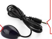
3.5mm jack, insert it into the specialized socket (3.5mm) to connect the IR receiver with the amplifier
